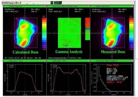
The detector reading, for each arc, is converted to a dose map and compared with the TPS (Eclipse) dose distribution (calculation grid of 0,25cm) and analysis with EpiQA
